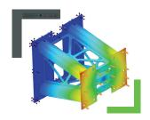
· With Creo Ansys Simulation, a higher-fidelity tool, you can automatically create mid-surface geometry for shell meshes; apply loads to create a pin and hole connection: and simulate unconstrained structures.
