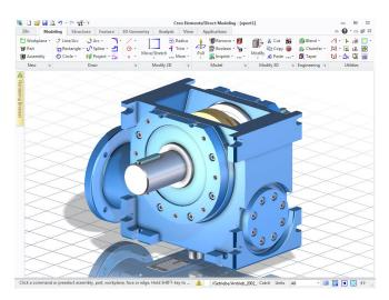
A direct approach makes 3D design creation and modification fast, easy, and flexible. You can rapidly evolve a product design in unpredictable and new directions when modifications cannot be anticipated in advance.
