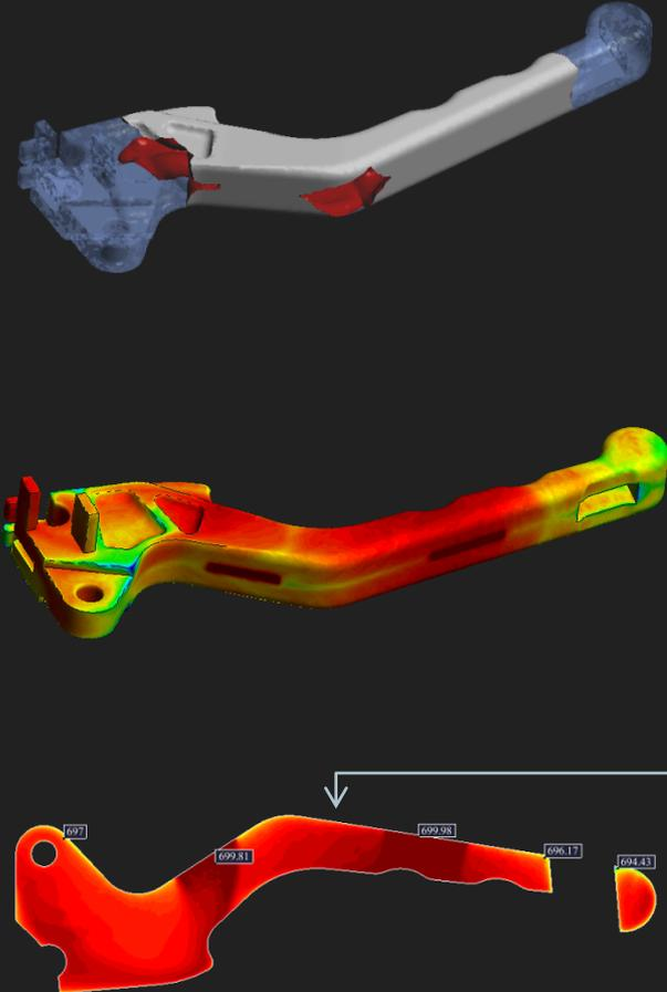
Front flow results show the filling material evolution. This visualization gives a preliminary idea of the filling time, and the way the part is filled. It's useful to decide the position of ingate and overflows to avoid air entrapment.
