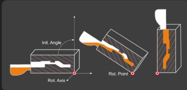
The rotation will be always following XYZ coordinate axis order; this means that if we select Y as axis of rotation, then the rotation will turn Z over X; if we select Z, then X will rotate over Y, and so on.
