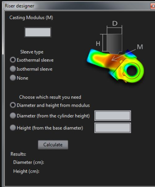
Solidification Modulus (Volume-to-area ratio) is the division between the casting Volume and the surface area (Units in meters). This option is useful in the riser designer wizard.
