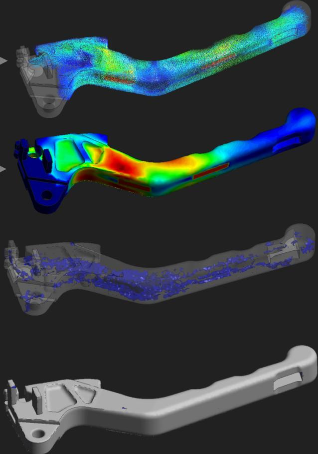
This option shows the vectors representation of the filling process. This way, we can detect turbulences and velocities. By clicking twice, It will show the velocities in iso-surface mode.
