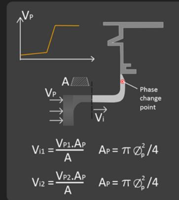
(4) Use first and second phase piston velocity if the piston and runner have been drawn. If not, it is possible to calculate the velocities using the attached formulas.
