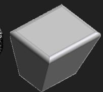
In case of radius at the selected ingate surface, the mesher can create an irregular ingate definition depending on the assigned element size.
