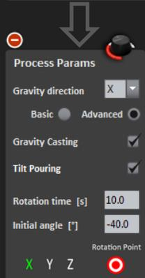
The initial angle must be negative. (e.g.  $-90^\circ$  or  $-45^\circ$ ) The final position is the actual position of the casting ( $0^\circ$ ).
