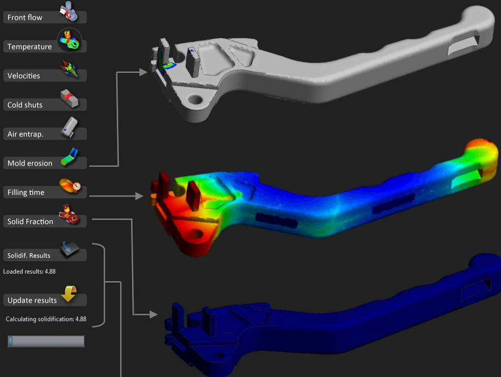
Mold erosion shows the areas with velocities exceeding 35 m/s, where there is high probability of mold degradation problems during the evolution of filling. By clicking twice, it's possible to change the maximum value.
