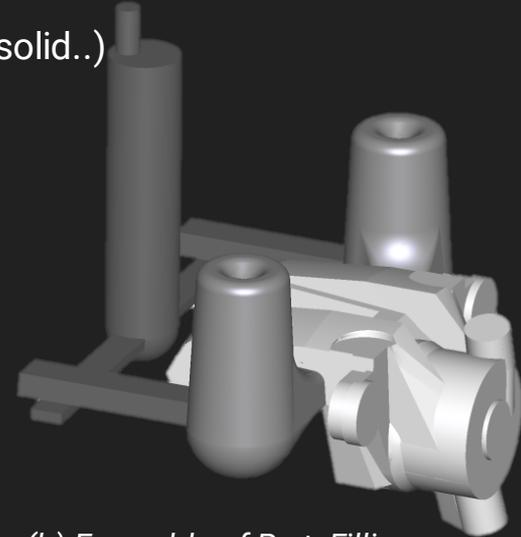
(b) Ensemble of Part, Filling system and risers.
